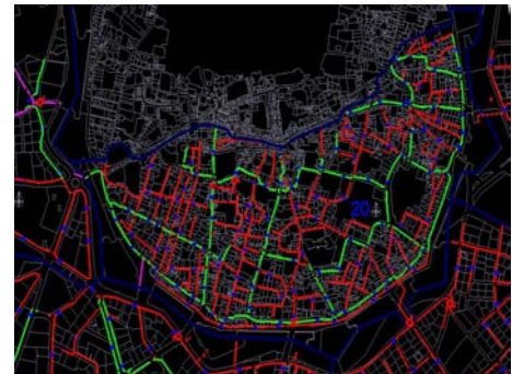
WBN pilot area DMA20 pipe network
